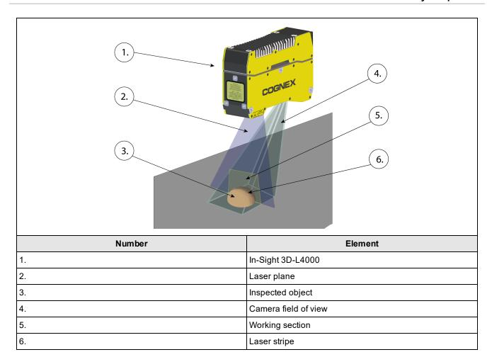
The vision system (1) projects a triangular laser plane (2) onto the object under inspection (3), illuminating the object's surface. The illumination of the laser plane determines the peak data of the raw 2D image and results in the 3D-L4000's laser stripe (6) within its field of view (4). The surface of the object determines the shape of the laser stripe, which provides the exact height profile information of the object; see the illustration below.
