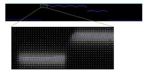
Factory calibration transforms the uncalibrated peak data into real-world coordinates and removes distortions such as camera lens and perspective. This creates a profile which represents the physical contours of the object. The image below shows a series of profiles.
