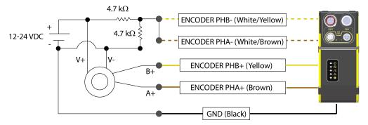
The image below shows the wiring of a differential encoder.
