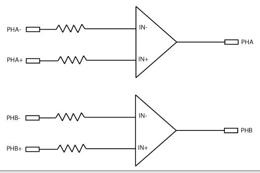
(i) Note: If you are using a Single-Channel Encoder, always connect to the 'PHA' input.
