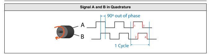
The distance per cycle is the physical distance that the conveyor system needs to travel to cause the encoder to output one full cycle. This distance can be calculated based on the dimensions of your encoder and the length of the image you want to acquire.
