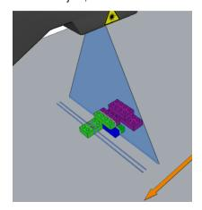
The following image illustrates the laser stripe as seen from the position of the vision system (on the left). The raw 2D image is what the vision system sees (on the right).
