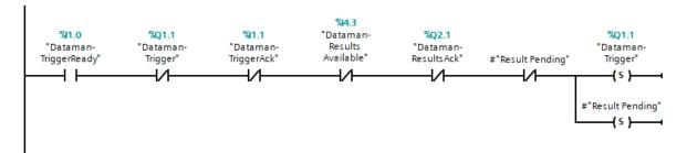
4. As soon as the results are available, clear the trigger signal and save a copy of the result data and set the results acknowledge signal.
