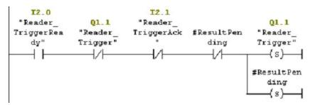
4. As soon as the trigger signal is acknowledged, clear the trigger signal.
