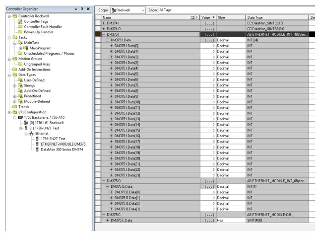
The tags are organized in three groups: Config "MyDM200:C", Input "MyDM200:I", and Output "MyDM200:O". You can ignore the Config tags (not used). The Input tags represent all the data being received (from the DataMan). The Ouput tags represent all the data being sent (to the DataMan).
