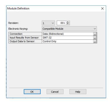
**Electronic Keying**: Defines the level of module type checking that is performed by the PLC before a connection is established.
