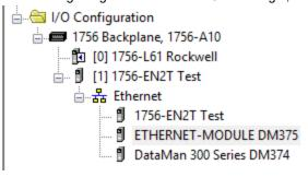
7. When the Generic Module is added to the I/O tree, RSLogix 5000 creates tags that map to the DataMan reader Input and Output Data (that is, the Input and Output Assembly Objects in the DataMan Reader). You can find these tags under the "Controller Tags" node of the project tree.
