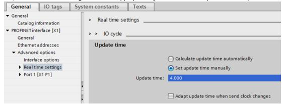
Note: The new GSD file has a faster cycle time, defaulting to 4 ms from 8 ms. While this shortens the network update interval, it also doubles the amount of PROFINET traffic from this device.
