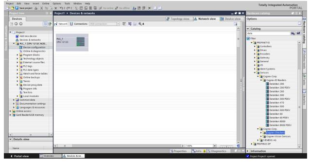
The HW Config tool automatically maps the DataMan I/O modules into the memory space.
