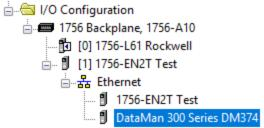
8. When the DataMan module is added to the I/O tree, RSLogix 5000 creates tags that map to the DataMan reader Input and Output Data (that is, the Input and Output Assembly Objects in the DataMan Reader). These tags can be found under the "Controller Tags" node of the project tree.
