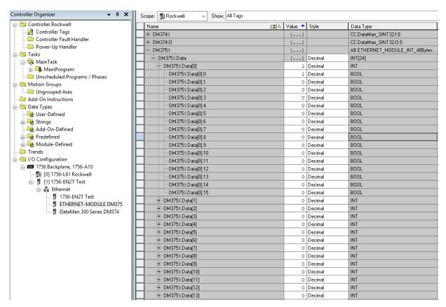
Output Assembly "Trigger": Bit 1 of word 0 of the Output Assembly. From the Output tag array for the DataMan select bit 1 of word 0.
