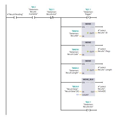
5. When the reader sees the result acknowledge signal, clear result acknowledge, clear the read pending coil, and signal that the read process is complete.
