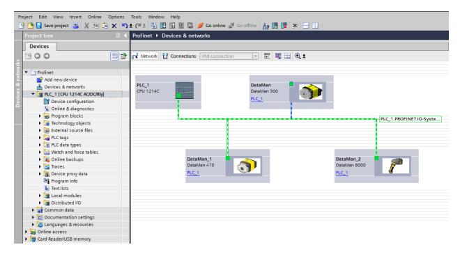
12. By default, the SIMATIC software maps the User Data and Result Data Modules to offset 256. This is outside of the default process image area size of 128. That is, data in these modules are inaccessible by some SFCs such as BLKMOV. As a solution, either remap the modules to lower offsets within the process image area or expand the process image area to include these modules.
