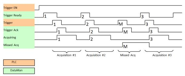
To force a reset of the trigger mechanism, set the *TriggerEnable* to False until *TriggerReady* is also set to False. Then, *TriggerEnable* can be set to True to re-enable acquisition.
