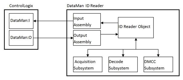
The *Input Assembly* and *Output Assembly* map various attributes (data) from the ID Reader object: The Input Assembly is the collection of DataMan reader data values sent to the PLC (PLC inputs); and the Output Assembly is the collection of data values received by the DataMan reader from the PLC (PLC outputs).
