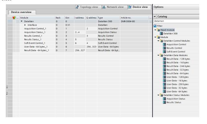
Note: Expanding the process image can have a performance impact on the PLC scan cycle time. If your scan time is critical, use the minimal acceptable module sizes and manually remap them down lower in the process image.
