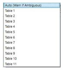
**Note**: The DM475 Verifier uses the X-dimension of the decoded symbol to deduce which table applies. If the X-dimension is outside of the range allowed in your application, results will be incorrect. To make sure that the verifier checks all the correct requirements for your application, select the Table in the GS1 General Specifications that applies to your application.
