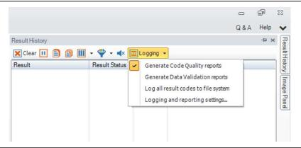
Note: The Code Quality report contains the results specific to verification when the verification feature key is installed and verification is enabled in the Setup Tool window. The Code Quality report contains the results and separate from the previous Code Quality results that Process Control Metrics (PCM) generate.
