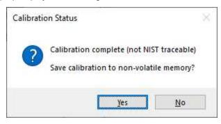
If you perform a successful calibration with a non NIST-traceable calibration symbol, no calibration date is recorded on the reports or displayed on the Main tab in the TruCheck window. Instead, The message reads "Calibration Complete (not NIST-traceable)".
