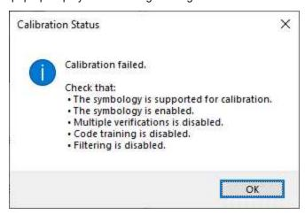
A failed calibration means that the calibration target was not detected. Ensure that:
