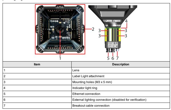
The image shows the back cover of the DataMan 475 and the functions of the indicator lights.
