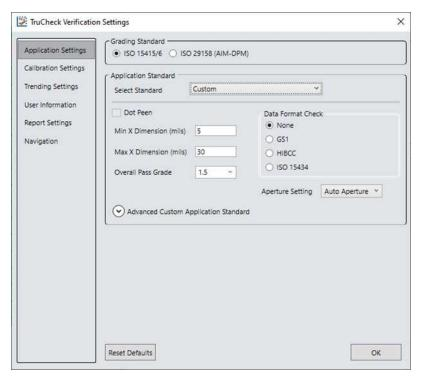
The **Custom** application setting options include **Advanced Custom Application Standard** option for the customization of grading by each individual quality parameter. The **Advanced Custom Application Standard** options allow you to select individual pass thresholds for each Quality Parameter for 1D and 2D symbologies. If a pass grade is selected for any of the Quality Parameters, the Overall Pass Grade, the Acceptance Criteria evaluation of Pass or Fail is overridden for that parameter.
