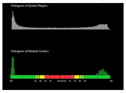
The horizontal axis on the **Histogram** represents the brightness level with the dark elements on the left side and the bright elements on the right side. As the element's brightness increases, the **Histogram** displays the element farther to the right of the **Histogram**. The height of each bar represents the number of elements with the same brightness associated with the elements' positions on the horizontal axis.
