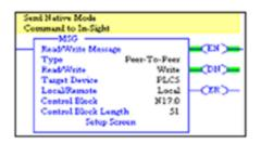
The Enable (EN) bit of the message instruction will be set to 1 when the input to the instruction is set high. The Done (DN) bit will be set to 1 when DataMan has replied that the DMCC command was received and executed with success. If the Error bit (ER) is enabled (set to 1), it indicates a problem with the message instruction. If an error occurs, click the Setup Screen for the MSG instruction. The Error Code will be shown at the bottom of the window.
